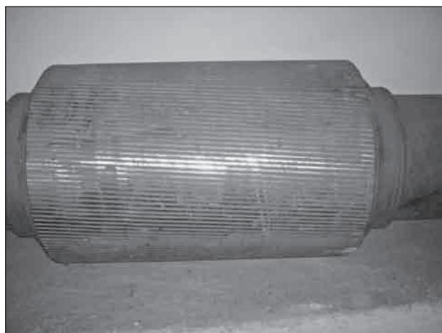
**Figure 1** Striated cylinder tool used to shred rubber waste
