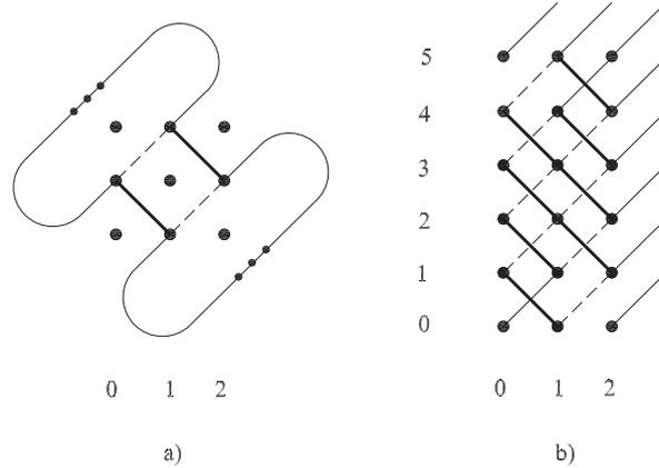
Figure 3: a) A switch that joins two parallel cycles into one cycle, b)  $p - 1$  switches that connect  $p$  parallel cycles into one (Hamiltonian) cycle
