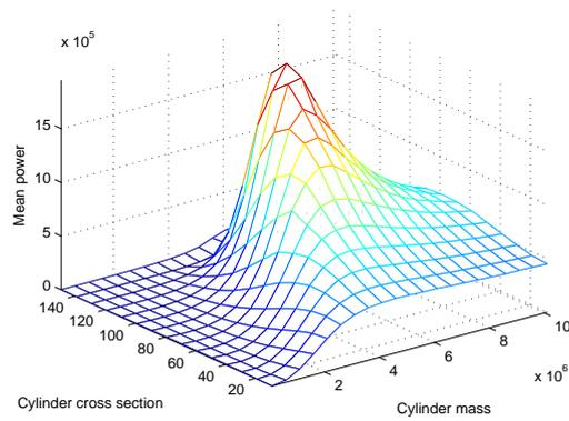
Figure 8: *Mean power versus annulus cross section and cylinder mass*
