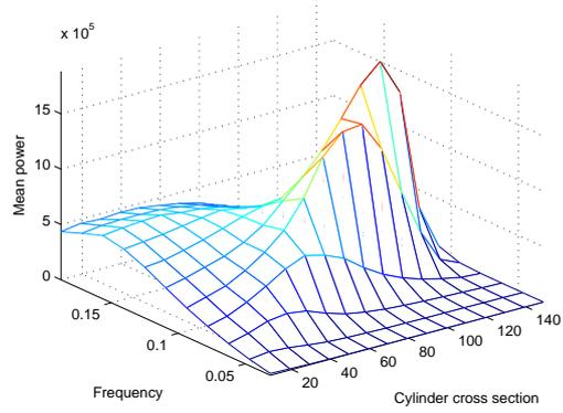
Figure 6: Mean power versus frequency and cylinder cross section
