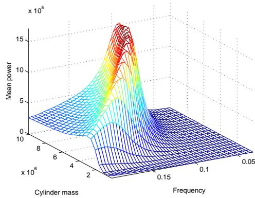
Figure 7: Mean power versus frequency and cylinder mass
