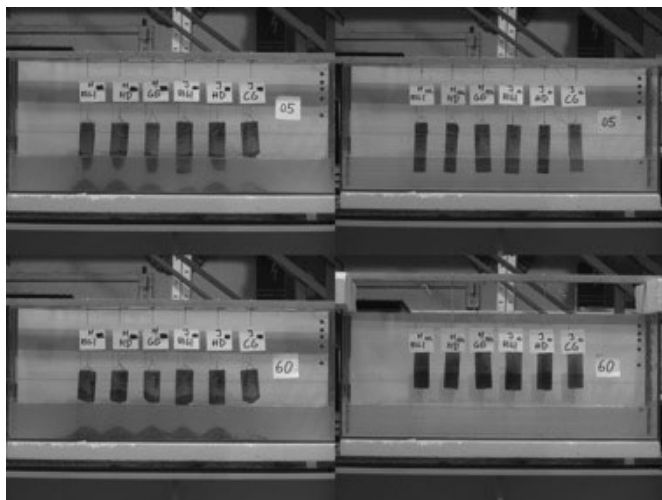
Figure 3. Test of resistance to water action according to Havlíček and Souček; the upper pictures visualize samples after 5 minutes, the lower ones after 60 minutes; the left side is without stabilization, while the right side was stabilized (0.5 wt% and 1 wt%).
