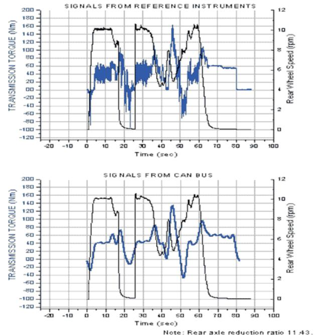
**Figure 12** Comparison between data provided through reference instruments (top) and CAN bus (bottom) for transmission torque and rear wheel rpm. Conditions: Bare tractor, acceleration and deceleration.
