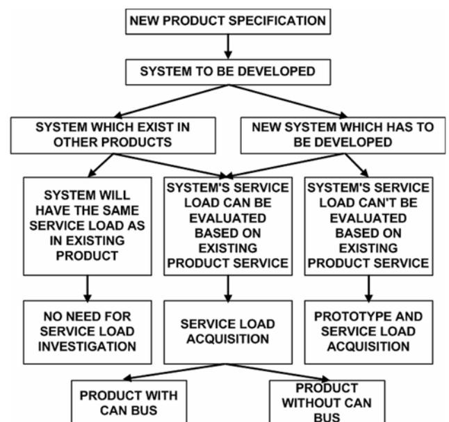
Figure 1 The new product development with reference to the knowledge of the service load
