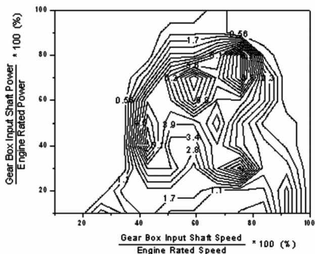
Figure 9 Transmission service load provided acquired through CAN bus and evaluated for direct comparison with matrix data related to PGN 65251
