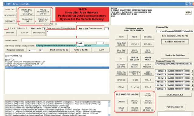
Figure 6 "Professional CAN Terminal" software – the main monitor page
