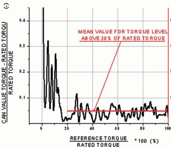
Figure 10 Analyses of the difference between CAN value for engine speed and reference engine speed (top) and CAN value torque and reference torque (bottom)
