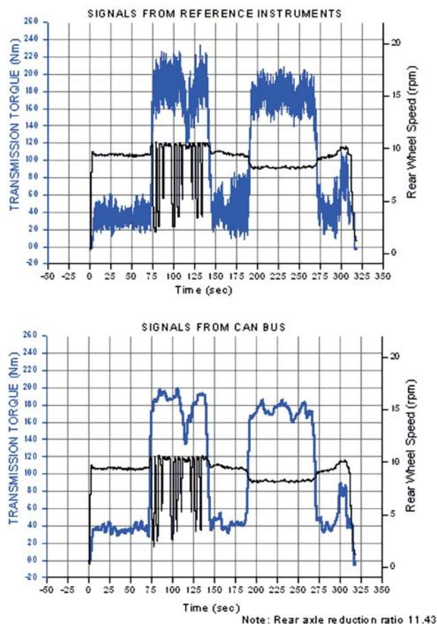
**Figure 11** Comparison between data provided through reference instruments (top) and CAN bus (bottom) for transmission torque and rear wheel rpm. Conditions: bare tractor, constant speed.
