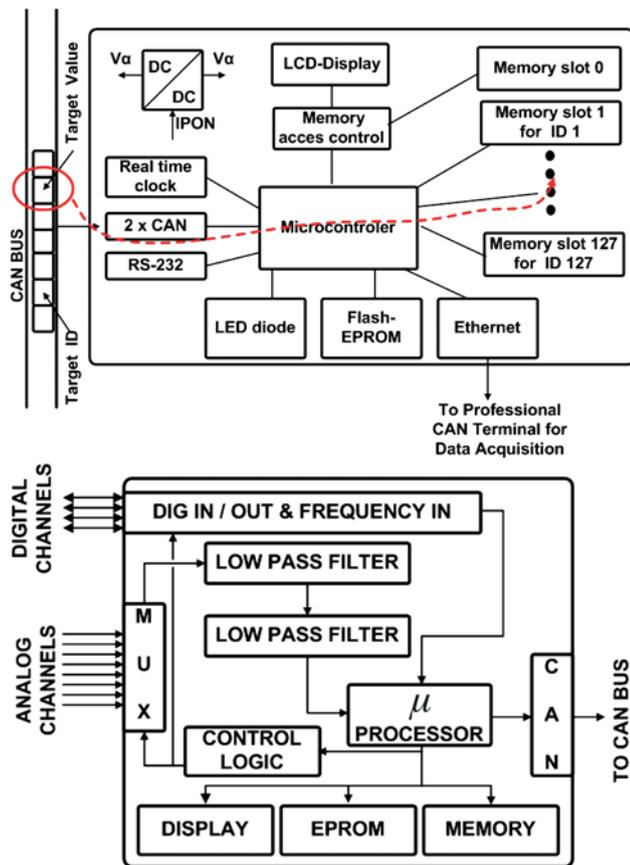
Figure 5 Configuration of the hardware components: top – WD (Watch Dog); bottom- EM (Extension Module)
