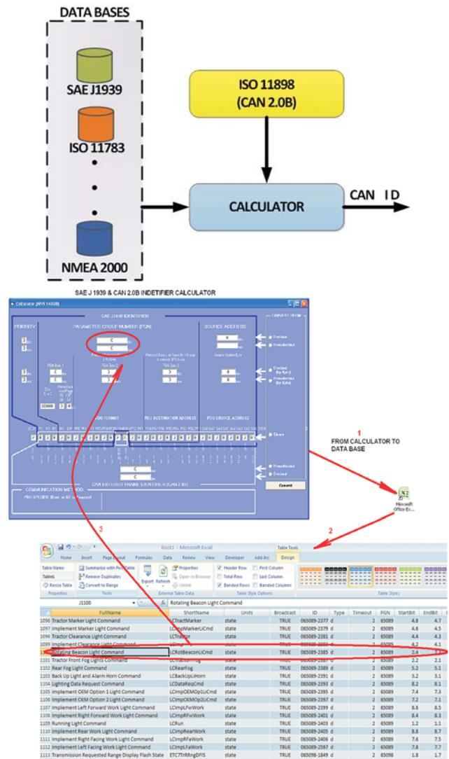
Figure 4 CAN Calculator; top – the software structure; bottom – the monitor page which provides support to the user to calculate CAN ID based on SAE J 1939 protocol
