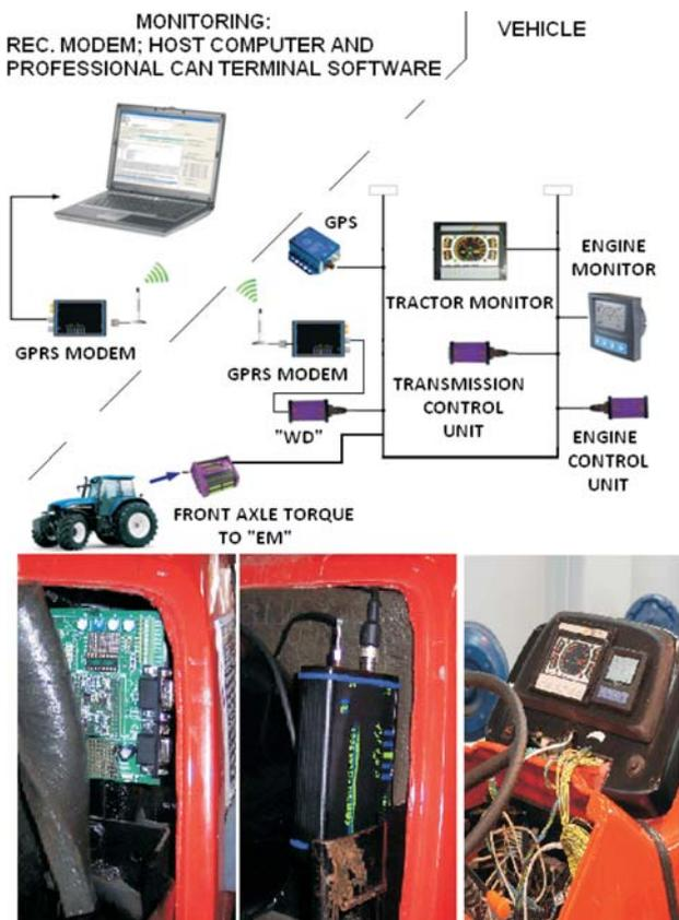
**Figure 7** System for service load data acquisition through CAN bus: top – configuration of the system, bottom left – EM built in the tractor; bottom middle – GPRS modem built in the tractor, bottom right – installation of the WD unit
