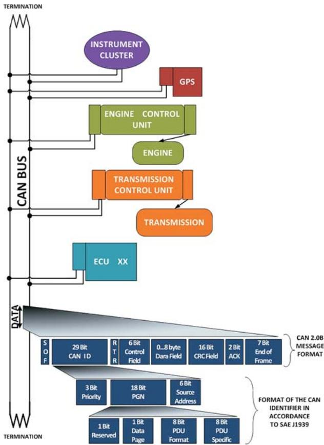
Figure 2 Common configuration of the vehicle's CAN bus (top) and the message format (bottom)
