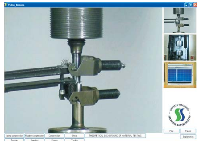
Figure 6 A screenshot of laboratory environment supported by three CCD cameras at the moment of specimen failure
