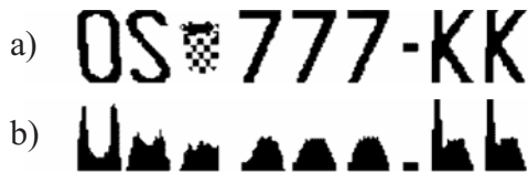
Figure 3 Vertical projection (b) of a binary license plate image (a)
