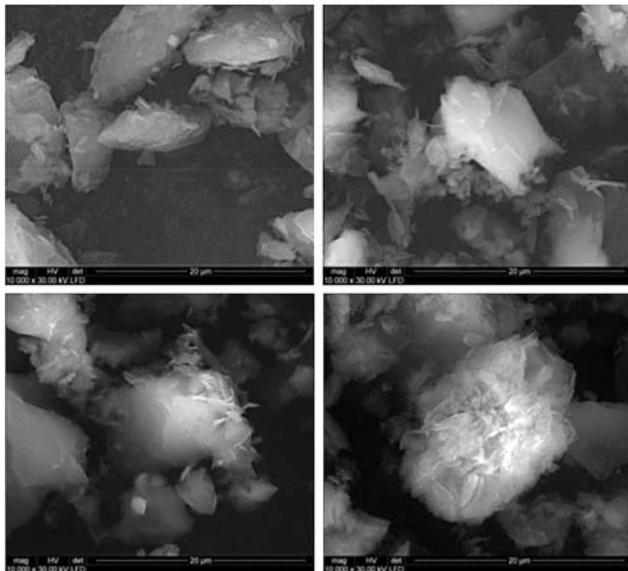
Figure 7 SEM pictures of hard coal showing different stages of their specific surface development
