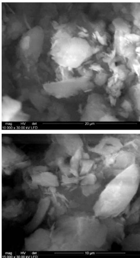
Figure 11 SEM pictures of brown coal comminuted with high-pressure water jet of 250 MPa showing different stage of their specific surface development
