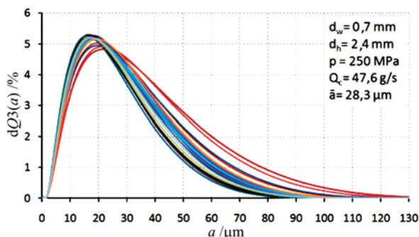
Figure 12 Distributions of charcoal grains fractions comminuted with water pressure of 250 MPa
