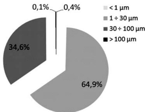
Figure 13 Quantitative contents of charcoal different fractions comminuted with high-pressure water jet ( $p= 250 \text{ MPa}$ )
