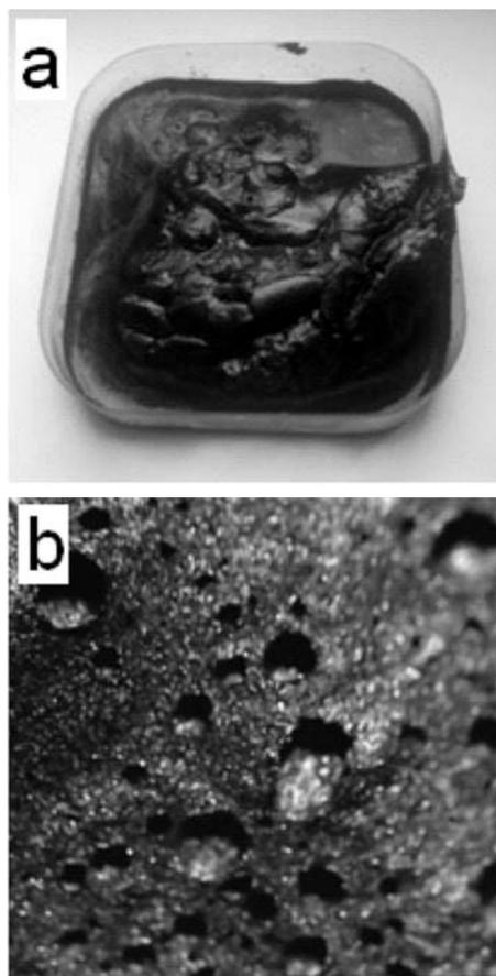
Figure 14 Air-dried charcoal mass (a) of great porosity (b), comminuted with high-pressure water jet ( $p= 250 \text{ MPa}$ )
