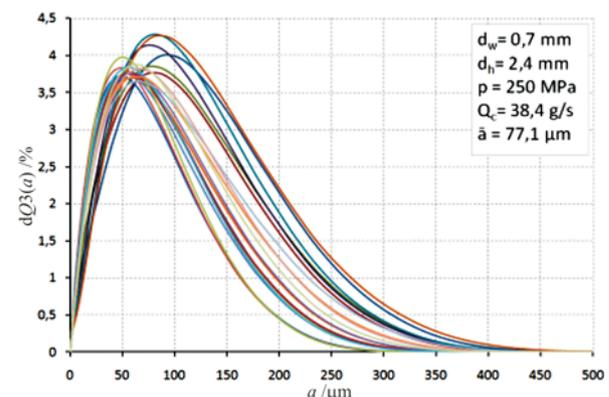
Figure 5 Distributions of hard coal particles fraction comminuted with water pressure of 250 MPa
