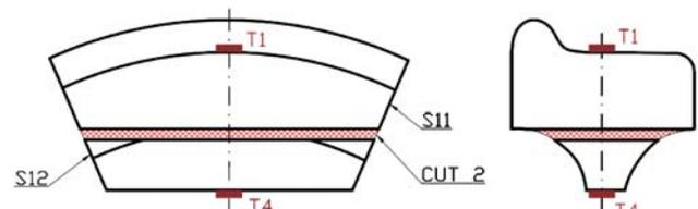
Figure 2 Location of strain gauge sensors
