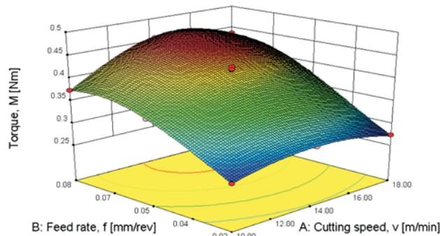
**Figure 11** The dependence of drilling torque on cutting parameters for "Brad & Spur" drill
