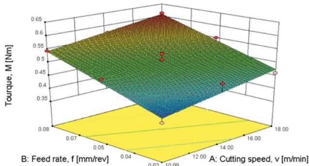
**Figure 10** The dependence of drilling torque on cutting parameters for Multi Constructional twist drill
