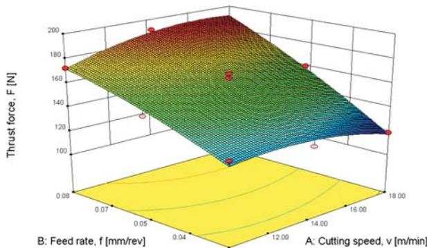
**Figure 8** The dependence of thrust force on cutting parameters for "Brad & Spur" drill
