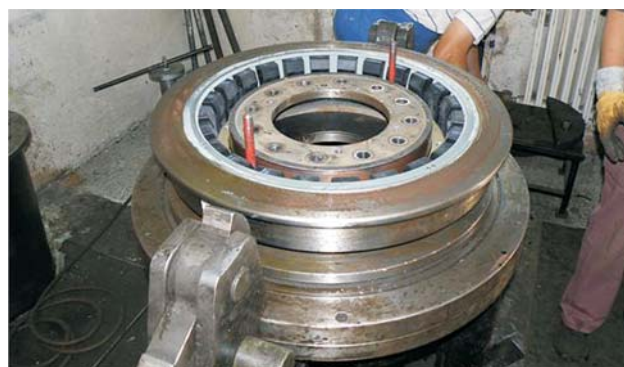
Figure 22 Resilient wheels (rubber pads installation)
