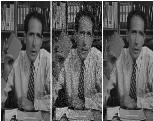
Figure 4. Denoising of video “Salesman” corrupted with noise \sigma = 20 using ATA method, frame 100; from left to right: original, noisy, denoised
