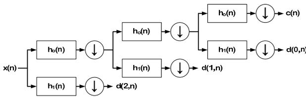
Figure 1. Wavelet filter bank
