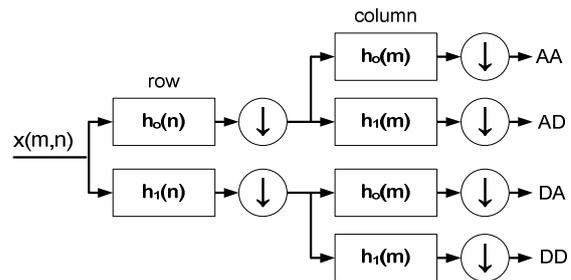
Figure 3. Separable 2D wavelet transform
