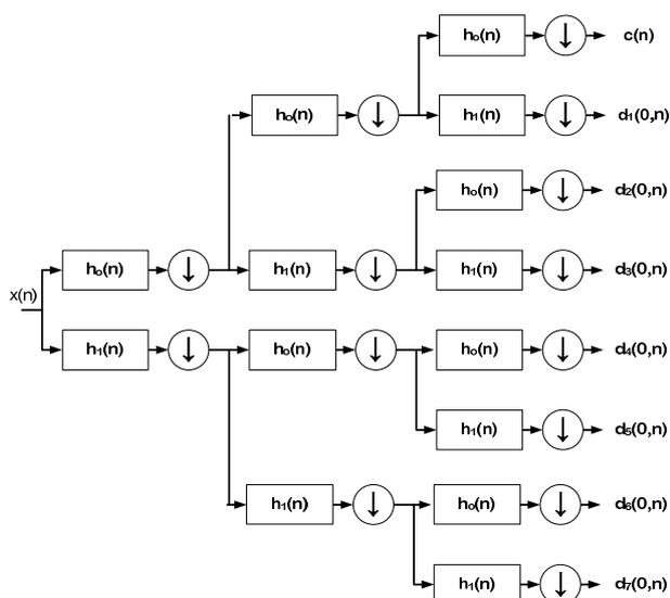
Figure 4. Wavelet packet transform
