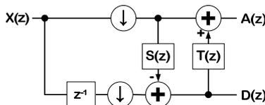
Figure 2. Lifting scheme
