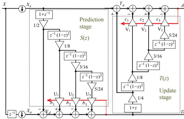
Figure 7. First stage of the lifting scheme with adaptive filters
