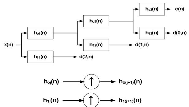
Figure 5. Stationary wavelet transform
