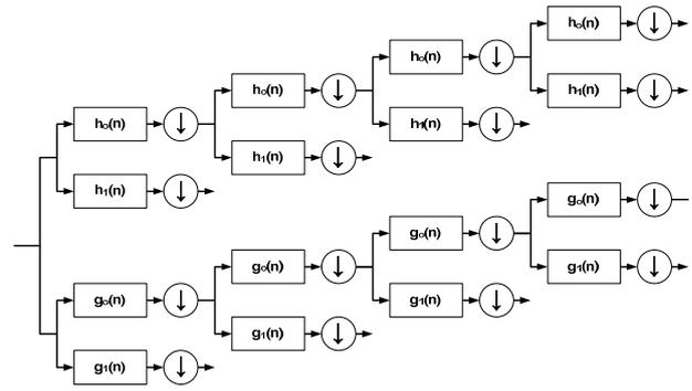
Figure 6. Realization of the dual – tree complex wavelet transform
