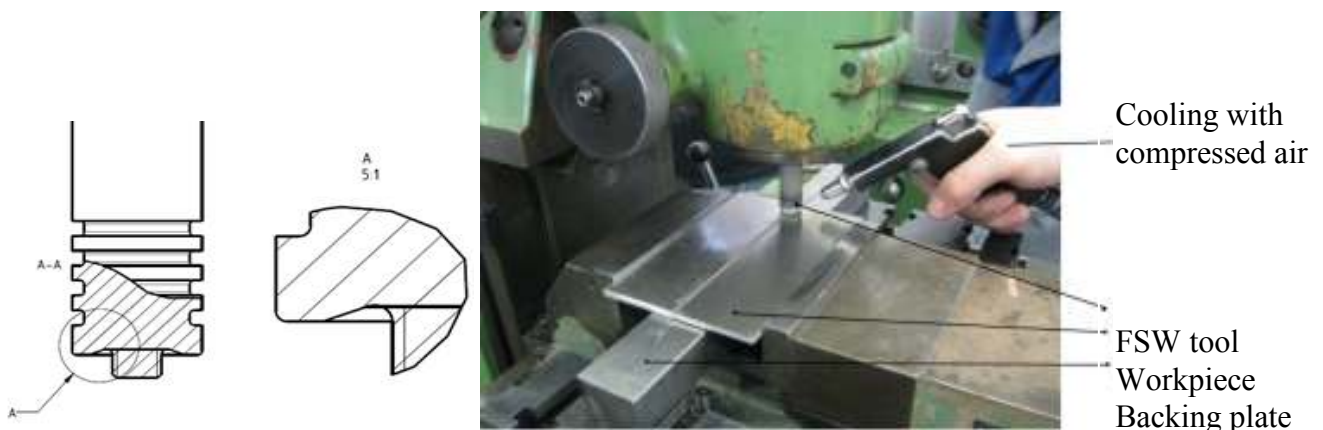
Figure 1 a) FSW tool geometry and b) experimental FSW.
