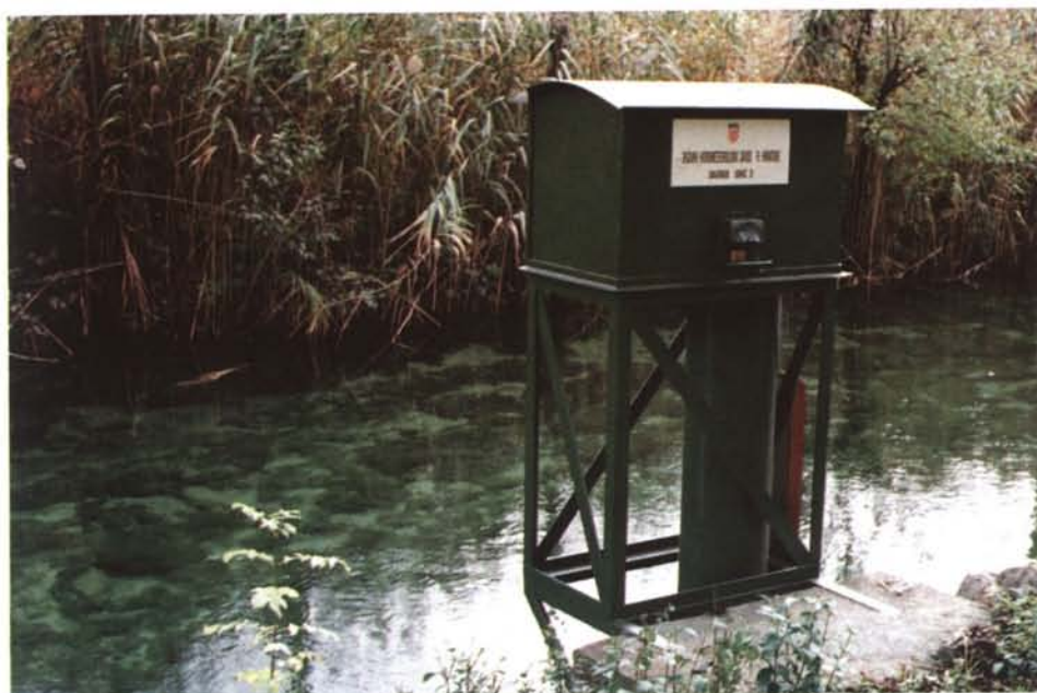
Fot. 5. Water stage recorder "Korana - Luketici" Fot. 5. Limnigraf "Korana - Luketici"
