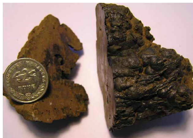
Figure 6: Black and shiny kidney shaped concretions and glassy needles in compact limonite (sample TLIM).
