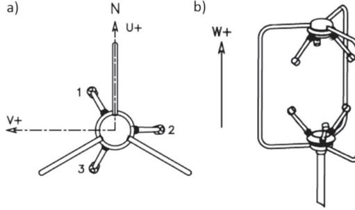
**Figure 4.** (a) Illustration of the WindMaster Pro sonic anemometer showing the coordinate system used in this study (top view) where the  $x$ -axis was aligned parallel to true north-south. Velocity components  $u_y$  and  $u_z$  were aligned with the true east-west and vertical, respectively. Numbers 1, 2 and 3 indicate the positions of anemometer sensors. (b) Position of ultrasonic anemometer on a boom, with the direction of vertical wind component is indicated.
