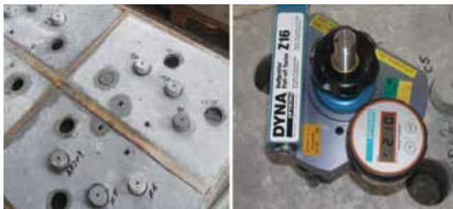
Figure 9. Reshaping system adhesion determined by pull off test
