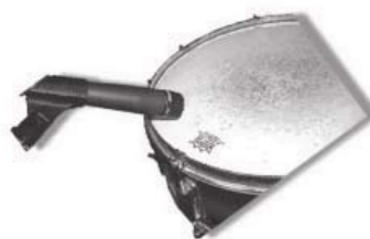
Figure 2. The snare drum recording. Shure SM57 is placed close to the edge, in parallel to the drumhead, and 6cm above it. The picture is taken with gratitude from [4].
