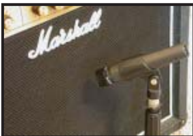
Figure 3. The placement of the microphone SM57 in front of the Marshall Valvestate 8040 combo amplifier.
