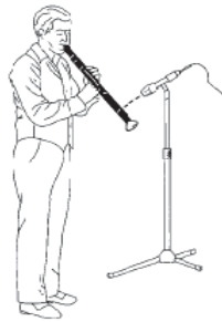
Figure 5. Clarinet recording. The microphone diaphragm axis is further off the instrument axis (on the picture to the right [4]).
