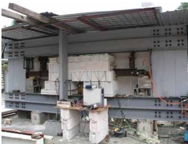
Figure 5. Test setup - furnace with a frame for loading steel elements
