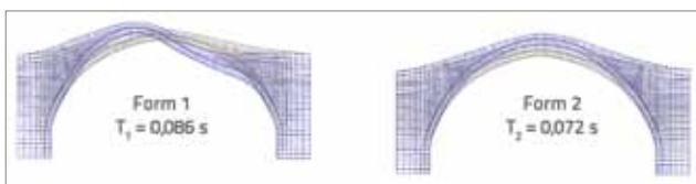
Figure 19. First two modes of free oscillation of the bridge
