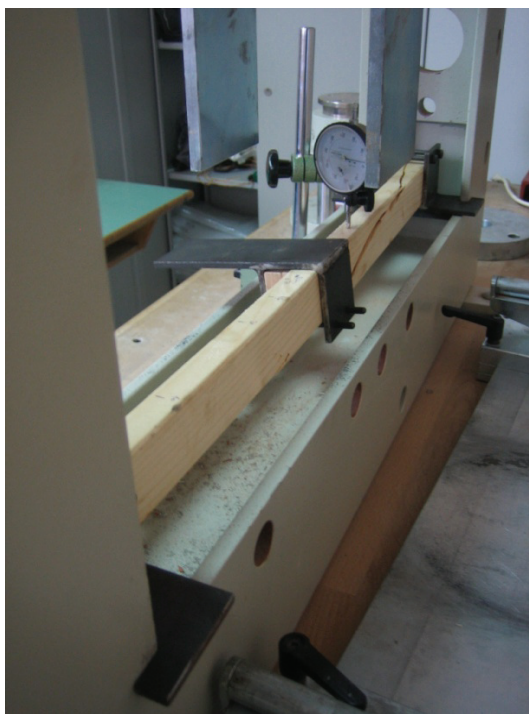
Figure 6 The failure of the sample
