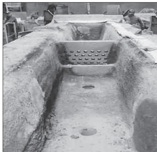
Figure 1 Tundish of the CC machine provided with the ceramic filter
