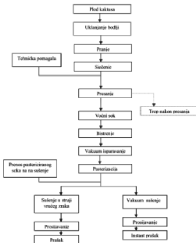
Slika 4. Shema tehnološkog postupka dobijanja praškaste forme kaktusa Figure 4. The scheme of technological process of powder form of fruit cactus
