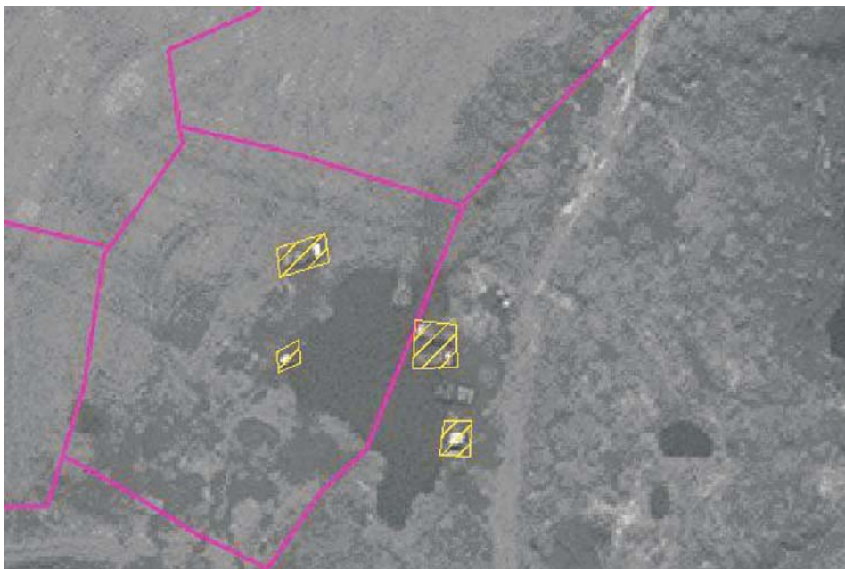
Fig. 7. Parcels Shared by Water Bodies Showing Encroachments in Hatchings.
