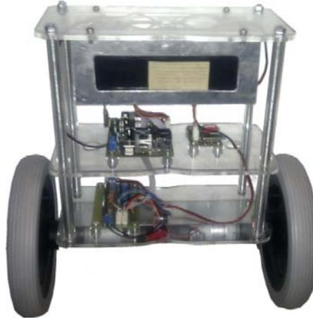
**Fig. 1** Self-balancing mobile robot
