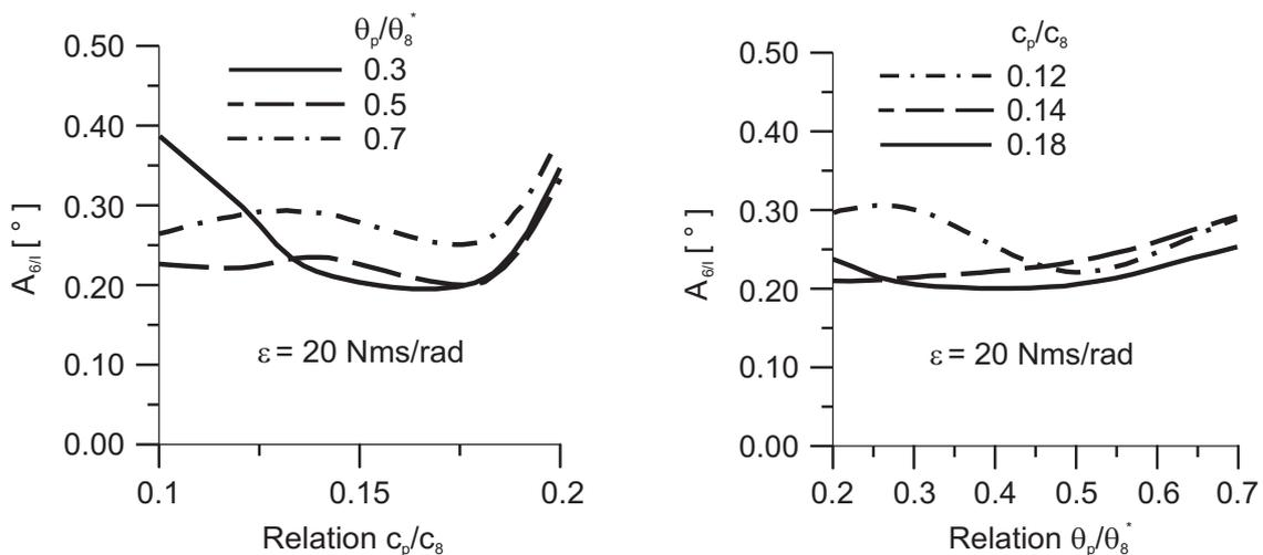
**Fig. 8** Diagram of the torsional vibration twist angle amplitudes ( $A_{6/1}$ ) at the engine pulley
