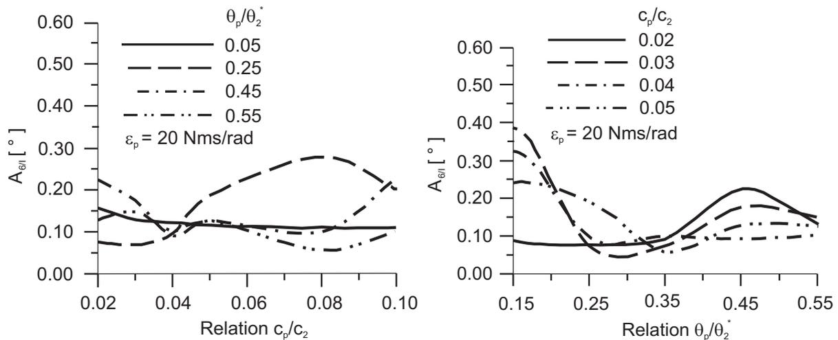
**Fig. 6** Diagram of twist angles of the torsional vibration amplitudes ( $A_{6/I}$ ) at the engine pulley ( $\theta_1$ ) depending on the relative stiffness and relative moment of inertia of the inertial mass of the balance weight damper
