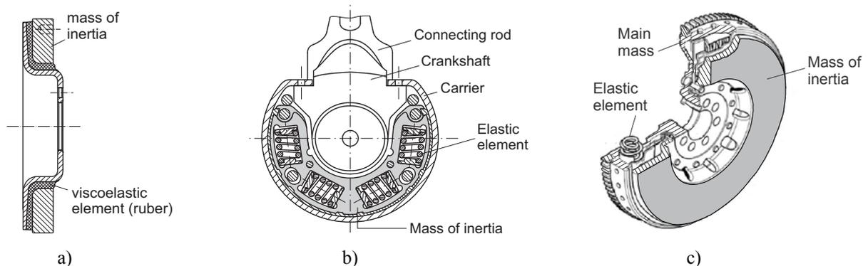
**Fig. 1** Three different TVDs for road vehicles IC engines
