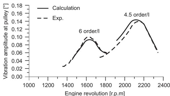
**Fig. 5** Diagram of calculated and experimentally obtained twist angles of the torsional vibration amplitudes at the pulley for the engine with an elastic TVD
