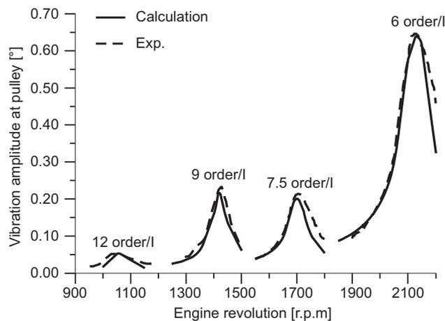
**Fig. 4** Diagram of calculated and experimentally obtained twist angles of the torsional vibration amplitudes at the pulley for the engine without a TVD
