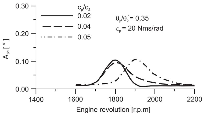
**Fig. 7** Diagram of twist angles of the torsional vibration amplitudes ( $A_{6/I}$ ) at the motor pulley ( $\theta_1$ )
