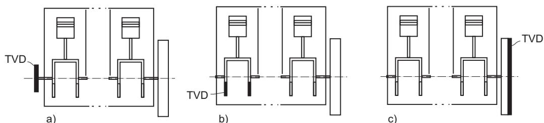
**Fig. 2** TVD mounting places in IC engines
