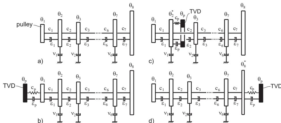
Fig. 3 Physical models of torsional vibration systems with different dampers
