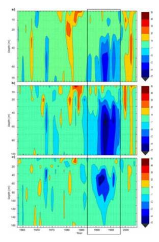
Fig. 5. Time evolution of vertical profiles (Hovmöller diagram) of MJJ standardized temperature anomaly at stations OS1 a), OS2 b) and OS3 c). Vertical scales differ between stations
