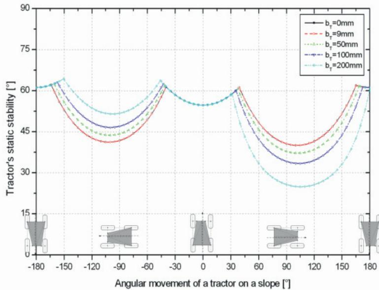
Figure 10. Simulating tractor's static stability in relation to the changes of the distance between the centre of gravity and tractor's symmetric plane
