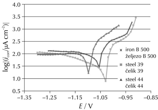
Fig. 4 – Potentiodynamic polarization curves for steel 44, steel 39, and iron B 500 in deaerated solution with  $c(\text{H}_2\text{SO}_4) = 1 \text{ mol L}^{-1}$  and  $c(\text{Cl}^-) = 10^{-3} \text{ mol L}^{-1}$ ,  $\text{pH} = 3.3 - 3.5$  without inhibitor (blank 2)
