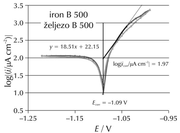
Fig. 6 – Potentiodynamic curves and Tafel extrapolations for iron B 500 in deaerated solution with  $c(\text{H}_2\text{SO}_4) = 1 \text{ mol L}^{-1}$  and  $c(\text{Cl}^-) = 10^{-3} \text{ mol L}^{-1}$ ,  $\text{pH} = 3.3 - 3.5$ , in presence of  $0.5 \text{ g L}^{-1}$  locust bean extract
