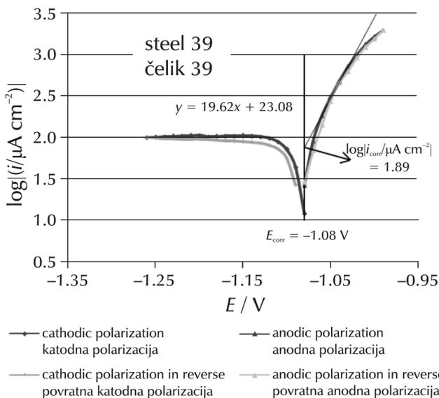
Fig. 5 – Potentiodynamic curves and Tafel extrapolations for steel 39 in deaerated solution with  $c(\text{H}_2\text{SO}_4) = 1 \text{ mol L}^{-1}$  and  $c(\text{Cl}^-) = 10^{-3} \text{ mol L}^{-1}$ ,  $\text{pH} = 3.3 - 3.5$ , in presence of  $0.5 \text{ g L}^{-1}$  locust bean extract
