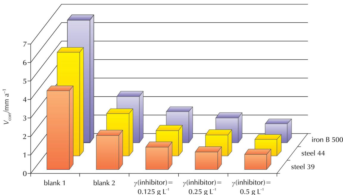
Fig. 8 – Diagram of corrosion rate for steel 39, steel 44 and iron B 500 in deaerated solution with  $c(H_2SO_4) = 1 \text{ mol L}^{-1}$  and  $c(Cl^-) = 10^{-3} \text{ mol L}^{-1}$ ,  $pH = 0.45$  (blank 1) and  $pH = 3.3 - 3.5$  (blank 2), with and without inhibitor
