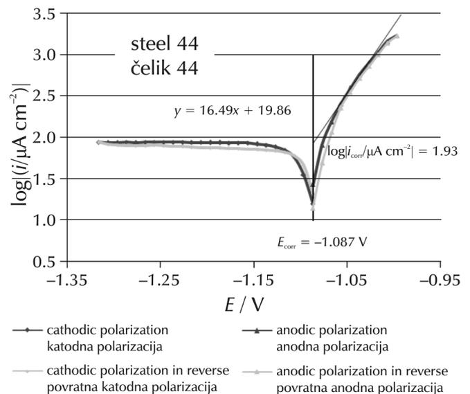
Fig. 7 – Potentiodynamic curves and Tafel extrapolations for steel 44 in deaerated solution with  $c(\text{H}_2\text{SO}_4) = 1 \text{ mol L}^{-1}$  and  $c(\text{Cl}^-) = 10^{-3} \text{ mol L}^{-1}$ ,  $\text{pH} = 3.3 - 3.5$ , in presence of  $0.5 \text{ g L}^{-1}$  locust bean extract
