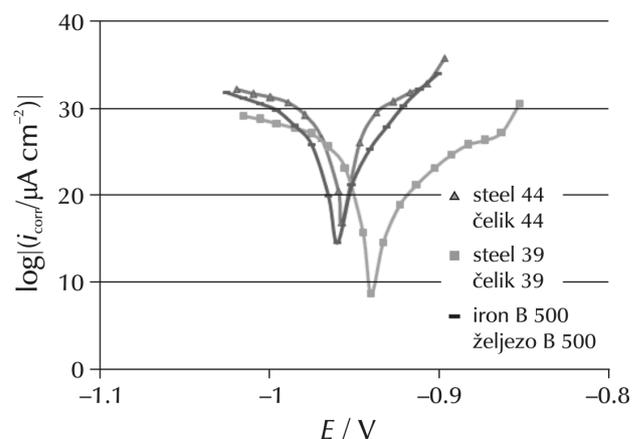
Fig. 3 – Potentiodynamic polarization curves for steel 44, steel 39, and iron B 500 in deaerated solution with  $c(\text{H}_2\text{SO}_4) = 1 \text{ mol L}^{-1}$  and  $c(\text{Cl}^-) = 10^{-3} \text{ mol L}^{-1}$ ,  $\text{pH} = 0.45$ , without inhibitor (blank 1)
