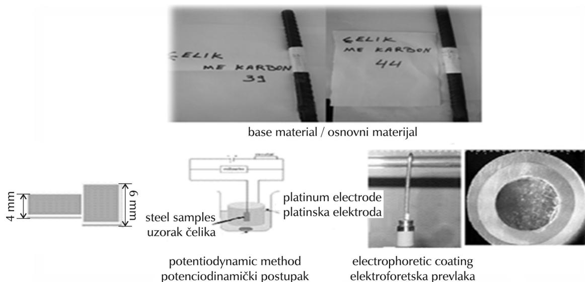
Fig. 1 – Preparation of samples for potentiodynamic measurements
