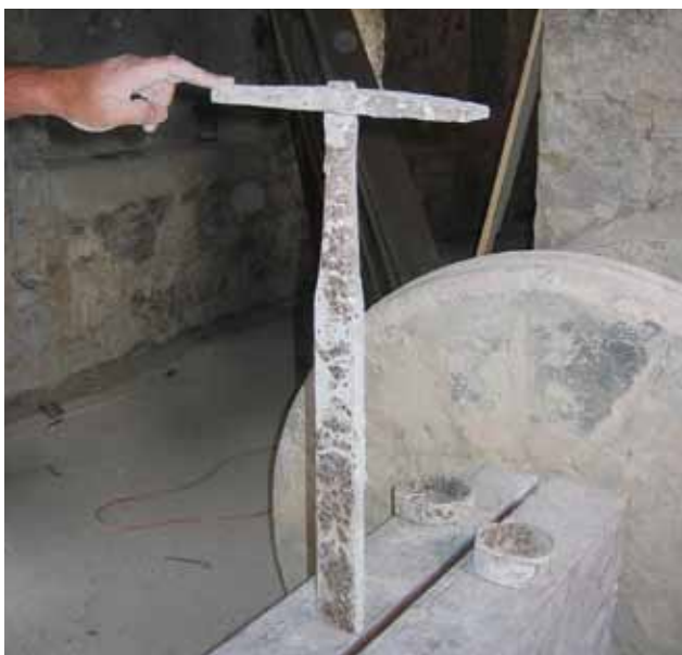
12 Jedini sačuvani dijelovi vretena: senj i dva obruča (foto: Sanja Buble, 2008.) The only preserved parts of the spindle: senj and two hoops (photo by Sanja Buble, 2008)
