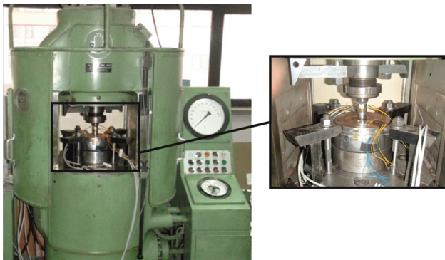
Figure 6 Sack&Kiesselbach hydraulic press with experimental tooling
