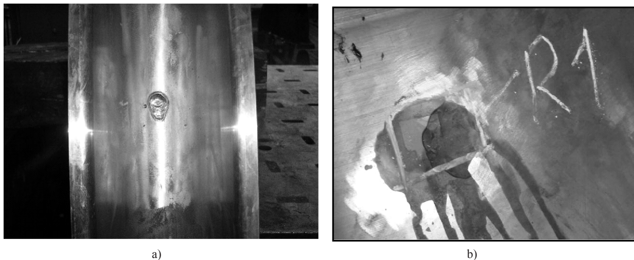
Figure 7. Sheaves with marked recovery spot by welding (a) and surface detail for replica (b)
