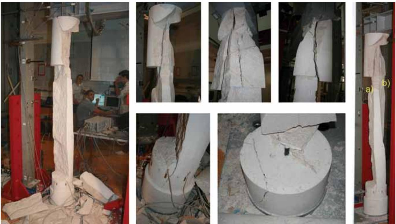
Figure 16. Sample K3 after failure [5]
