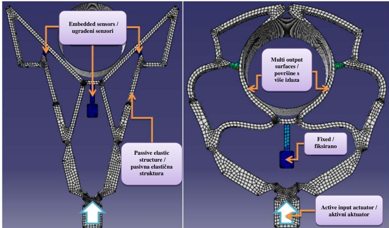
**Figure 3.** The main features of the adaptive gripper
