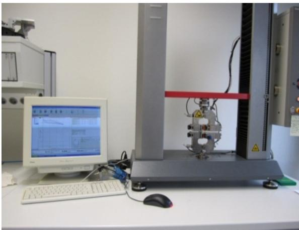
**Figure 6.** Experimental setup for ProLine material-testing machine
