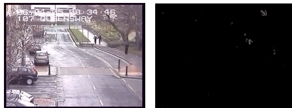
(a) Frame from the illumination invariance video sequence (b) Laplacian of Gaussian wavelet-based scene segmentation applied on a video frame we used to demonstrate its illumination invariance properties
