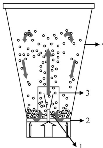
Fig. 1 – Schematic drawing of a bottom spray fluid bed equipped with a wurster insert, (1) spraying nozzle, (2) air distribution plate, (3) wurster insert, (4) expansion chamber. The gray colored arrows indicate the particle flow, the white colored arrows indicate the fluidizing inlet air flow.
