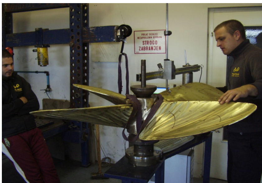
Slika 5. Postupak mjerenja vijka Prop Scan tehnologijom [1] Figure 5 Procedure for measuring a propeller using the Prop Scan technology [1]
