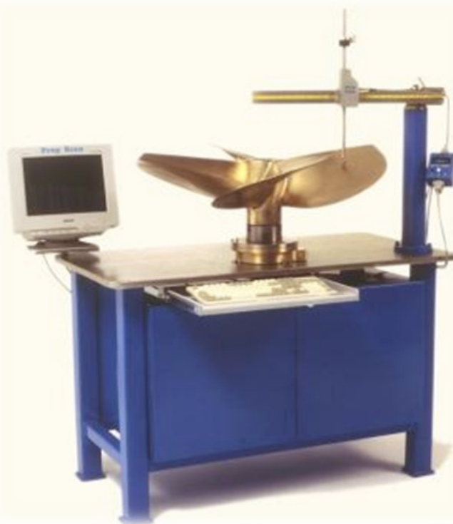
Slika 2. Prop Scan sustav za ispitivanje vijka Figure 2 Prop Scan system for testing propellers
