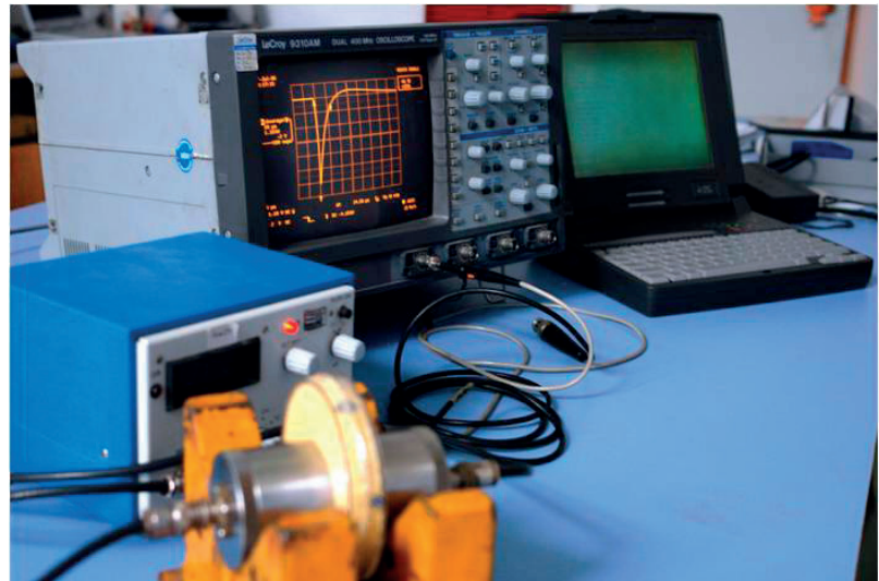
Figure 1. Determination of unwanted foreign bodies using low intensity ultrasound (Brnčić et al, 2009)
