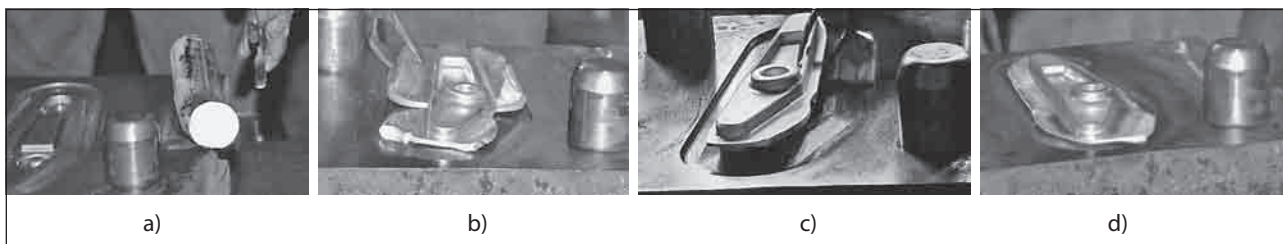
Figure 6 The product shape after the following forging stages: a) bending, b) initial operation, c) trimming, d) final operation
