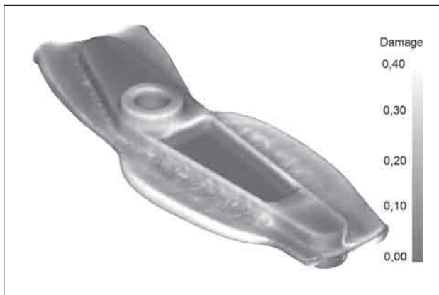
Figure 4 Distribution of damage criterion according to Cocroft-Latham at final stage of initial forging operation
