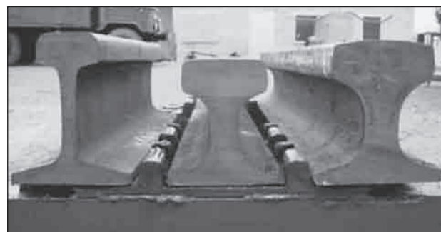
Figure 3 Types of rail profiles
