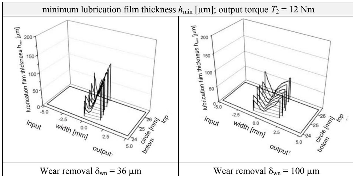
Fig. 11 Minimum lubrication film thickness for different wear removals
