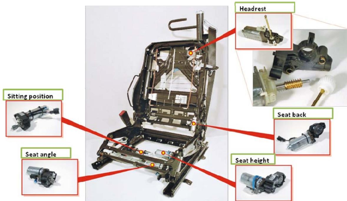
Fig. 1 Crossed helical gears in drive units for seat adjusting in BMW E46 C [6]
