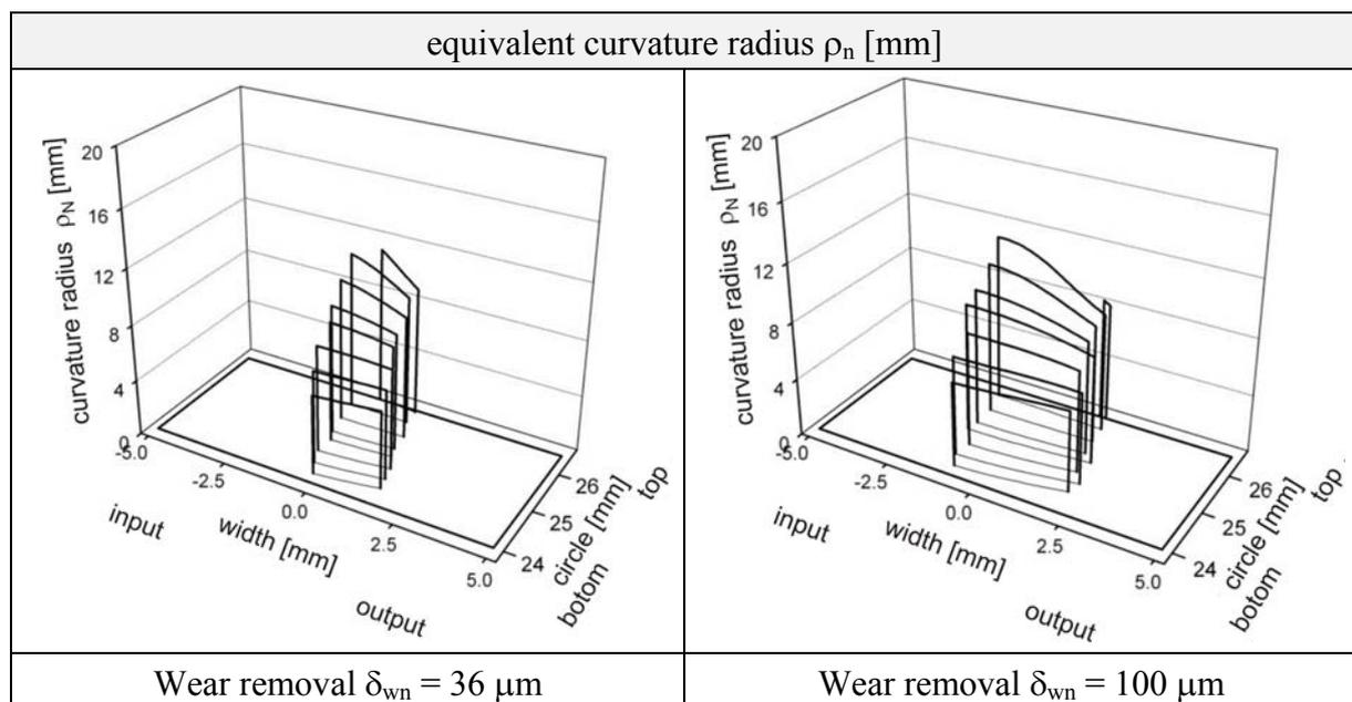
Fig. 7 Equivalent curvature radius for different wear removals
