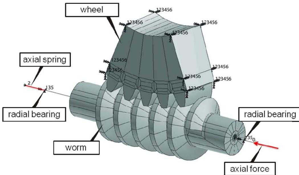
**Fig. 4** Worm and wheel – constraints of the degrees of freedom
