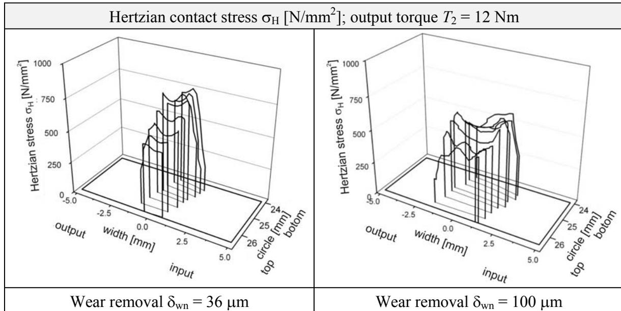
Fig. 8 Hertzian contact stress for different wear removals
