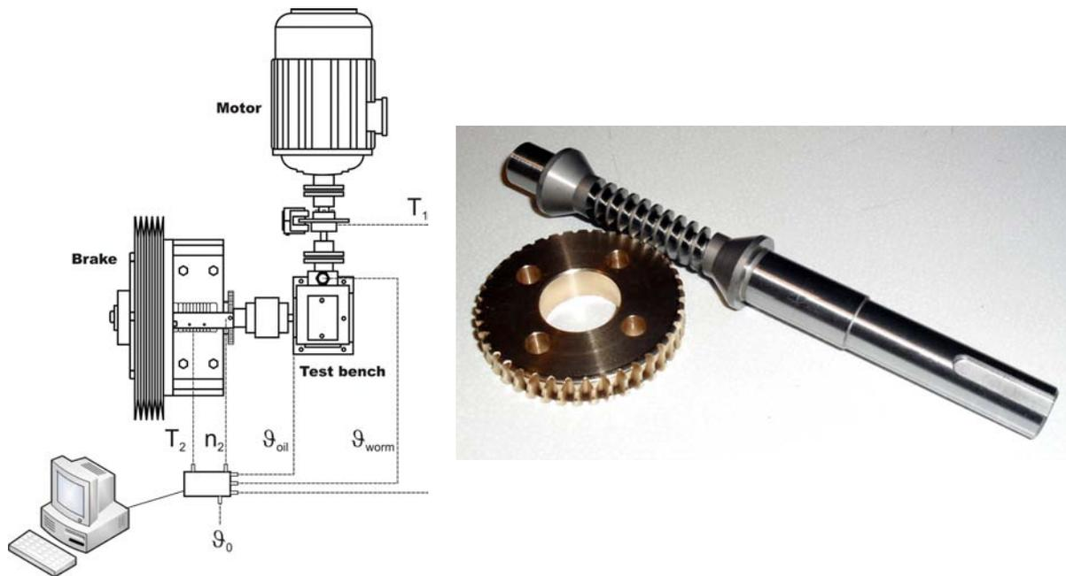
Fig. 2 Test bench and test gear pair
