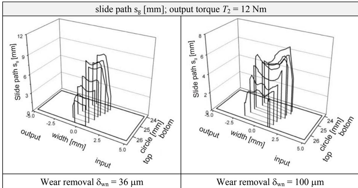
Fig. 10 Slide path for different wear removals
