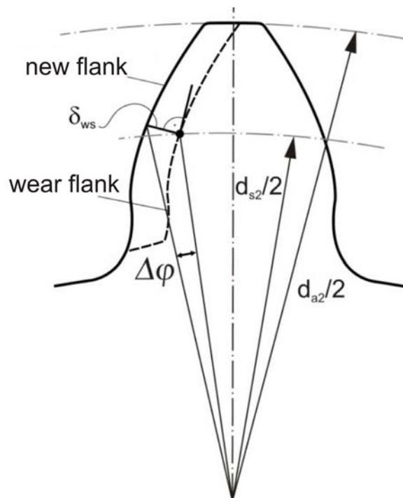
Fig. 12 Transverse section of a wheel with and without wear
