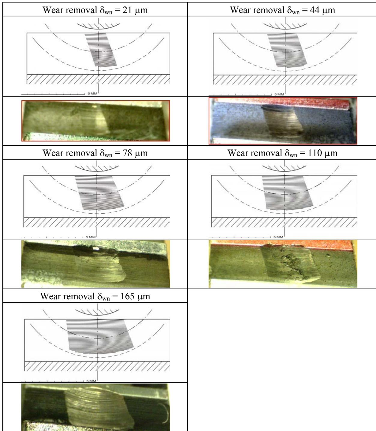
**Fig. 6** Experimental and FEM results of wear in wheel flanks for different wear removals
