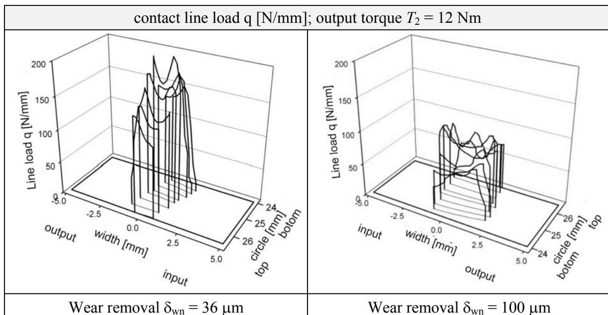
Fig. 9 Contact line load for different wear removals
