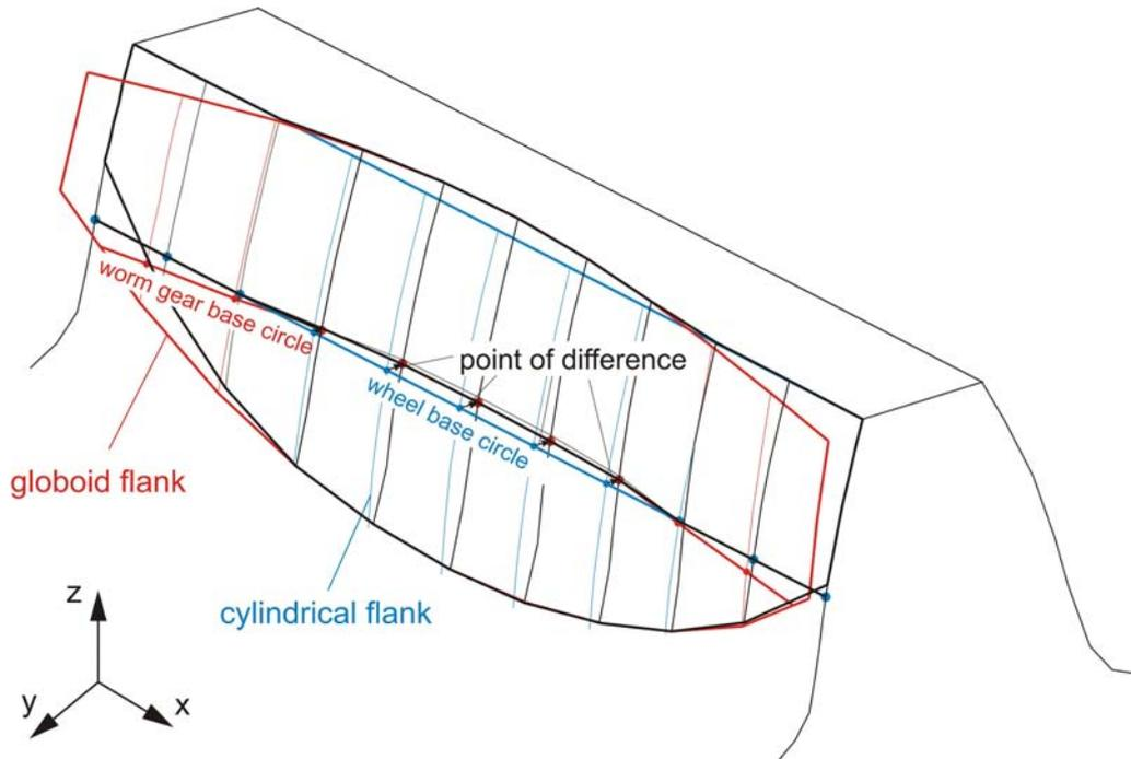
**Fig. 13** Difference between the points of the cylindrical and globoid flank on base circle
