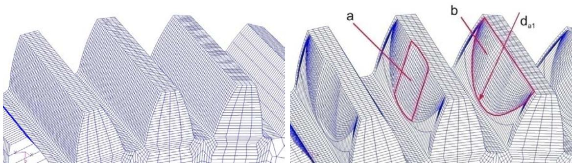
**Fig. 5** FEM model of crossed helical gear in new and in wear state (a – wear surface, b – maximal contact surface,  $d_{a1}$  – addendum circle of worm)
