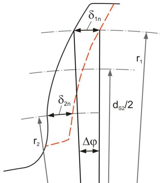
**Fig. 14** Wear removal as a function of the tooth height
