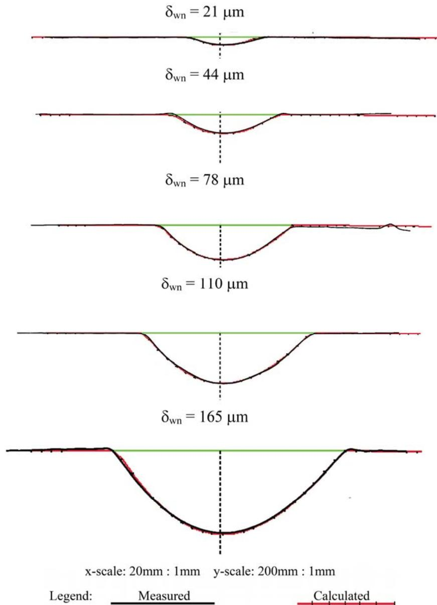
**Fig. 15** Comparison of calculated and measured wear removals
