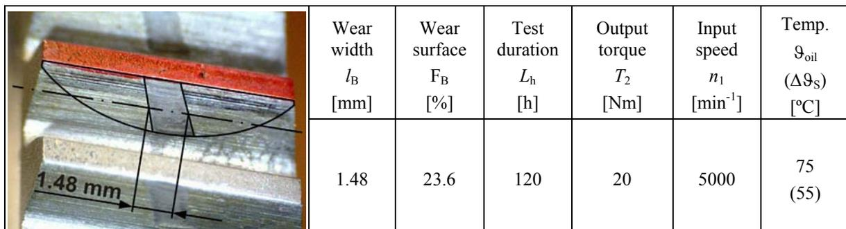
Fig. 3 Wear on tooth flank of the wheel
