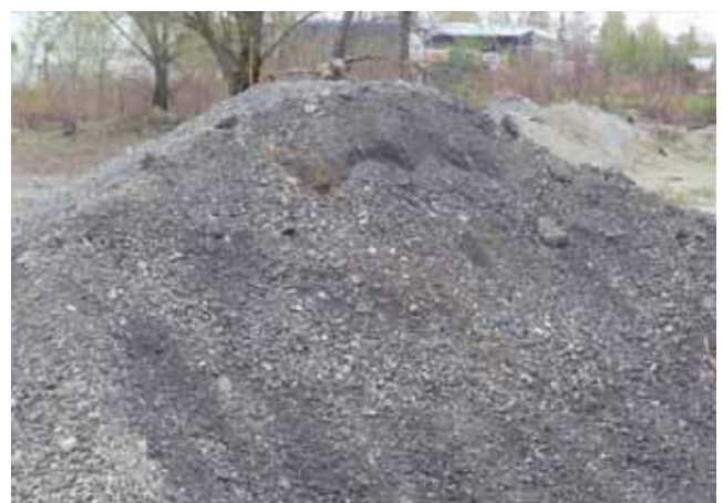
Figure 1. Recycled asphalt stockpile
