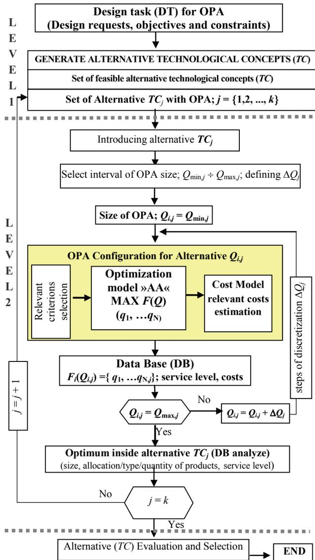
Figure 2 The procedures for OPA design
