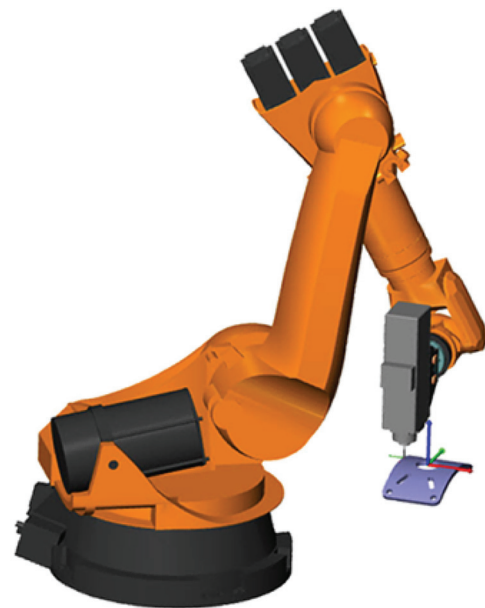
Figure 2 After applying the method of rotating the end-effector around tools symmetry axis the part can be machined
