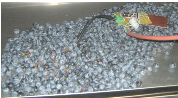
Figure 12a Setting up the interdigital sensor, A channel
