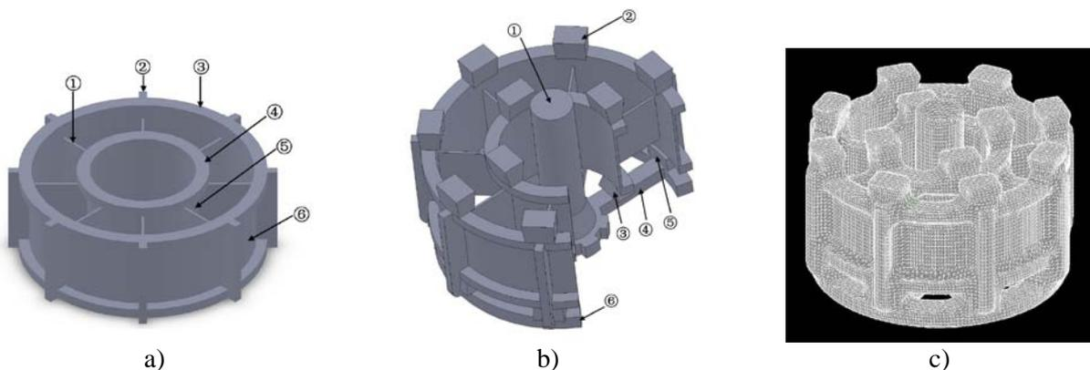
Figure 1. a) A schematic picture of titanium casting; b) Pouring system designed for casting; c) FEM Mesh of Casting and its pouring system.
