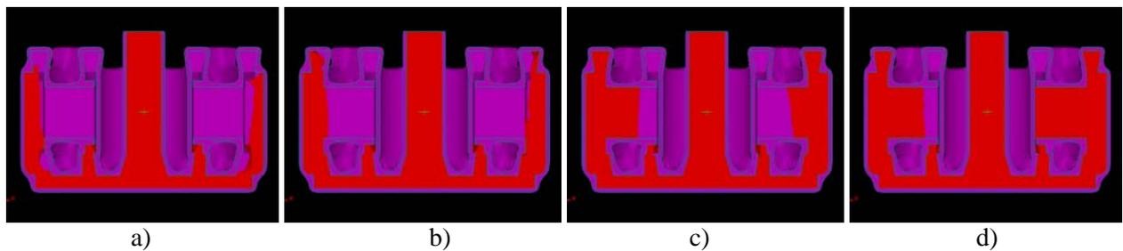
Figure 7. Melt free surface in the thin-walled ribs at 150rpm: a)  $t=0.46s$ ; b)  $t=0.63s$ ; c)  $t=0.70s$ ; d)  $t=0.72s$ .
