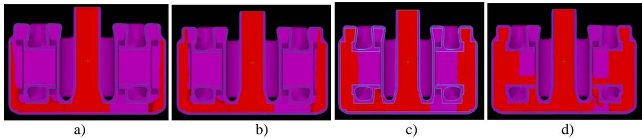
Figure 8. Melt free surface in the thin-walled ribs at 500rpm: a)  $t=0.23s$ ; b)  $t=0.31s$ ; c)  $t=0.56s$ ; d)  $t=0.63s$ .
