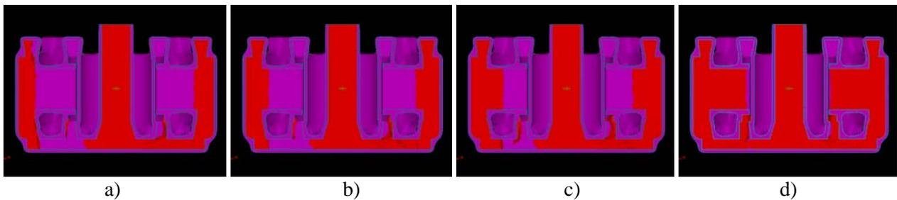
Figure 6. Melt free surface in the thin-walled ribs at 300rpm: a)  $t=0.53s$ ; b)  $t=0.57s$ ; c)  $t=0.59s$ ; d)  $t=0.66s$ .
