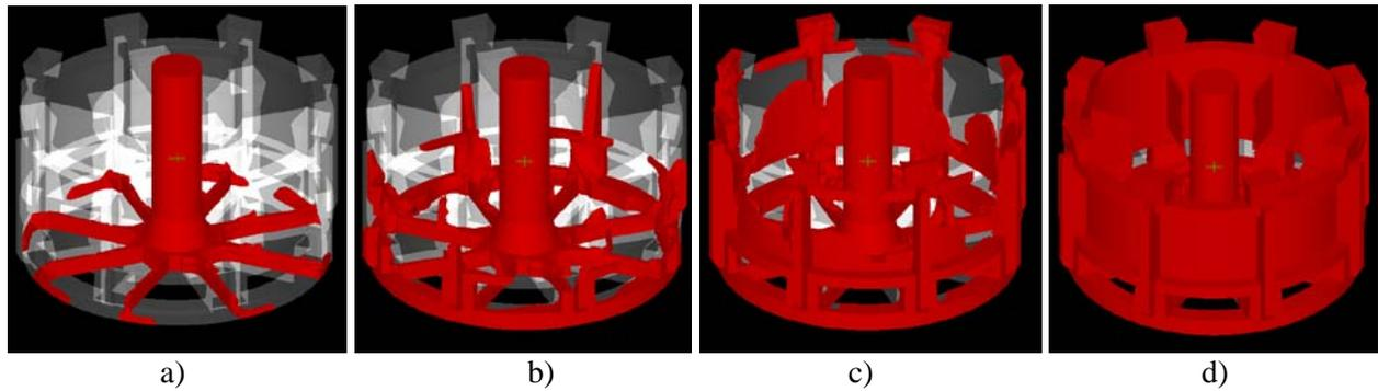
Figure 2. Melt filling state in the cavity during vertical centrifugal casting process: a)  $t=0.16s$ ; b)  $t=0.26s$ ; c)  $t=0.42s$ ; d)  $t=0.61s$ .
