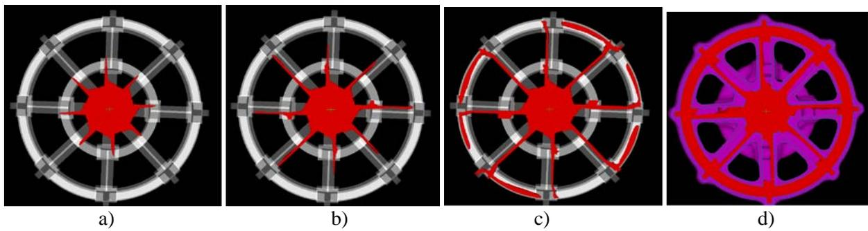
Figure 5. Melt free surface in the radial runner at 500rpm: a)  $t=0.13s$ ; b)  $t=0.14s$ ; c)  $t=0.16s$ ; d)  $t=0.55s$ .
