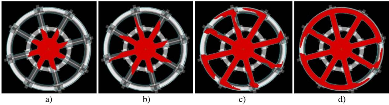
Figure 4. Melt free surface in the radial runner at 150rpm: a)  $t=0.16s$ ; b)  $t=0.19s$ ; c)  $t=0.28s$ ; d)  $t=0.36s$ .
