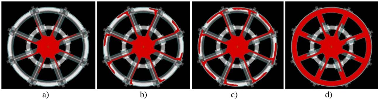
Figure 3. Melt free surface in the radial runner at 300rpm: a)  $t=0.14s$ ; b)  $t=0.16s$ ; c)  $t=0.17s$ ; d)  $t=0.61s$ .
