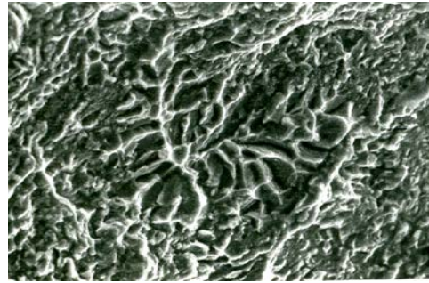
Figure 5 Character of the dendrites deformation \alpha of the solid solution and eutectics.
