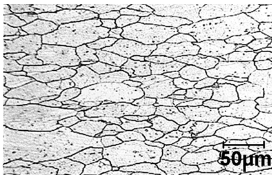
Figure 6. Microstructure of welding tip made by forming of CuCoBe
