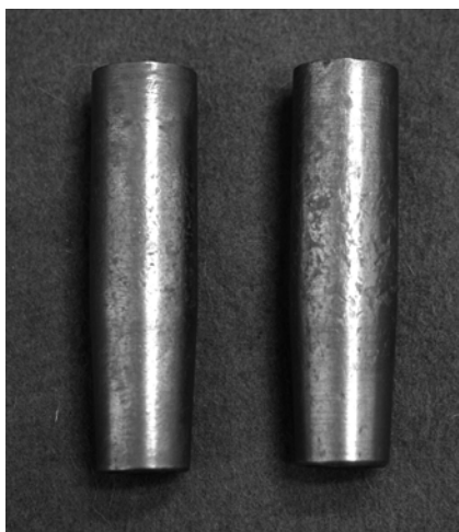
Figure 1. Welding tips for metallographical analysis from CuCr1Zr material
