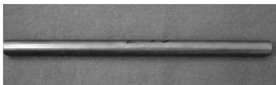
Figure 2. Bar workpiece for production of CuCoBe welding tips (ø 16 mm × 300 mm)
