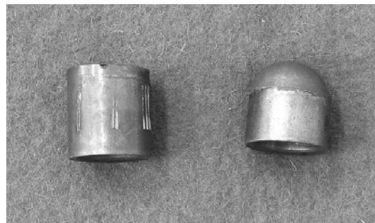
Figure 3. Welding tips for metallographical analysis from CuBe2 material
