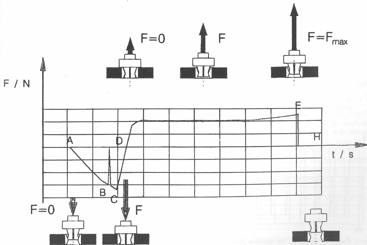
Figure 2 Time sequence of the force of joining and separating the examined attachment
