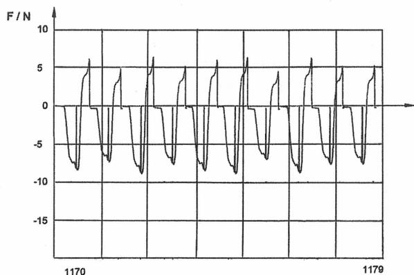
Figure 7 Change of the retention force with added saliva - loading cycles 1170 - 1179.
