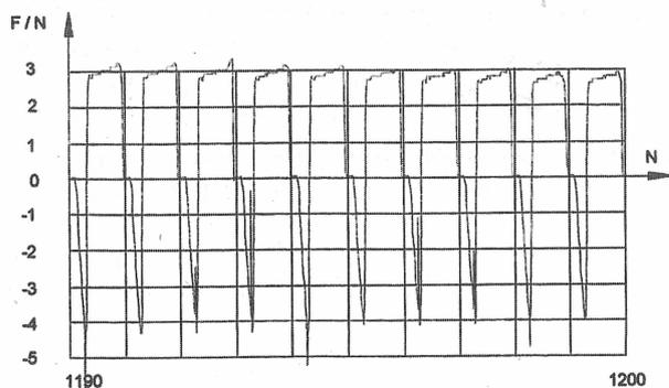
Figure 4 Results of measuring the retention force with dry touching surfaces - loading cycles 1190-1200
