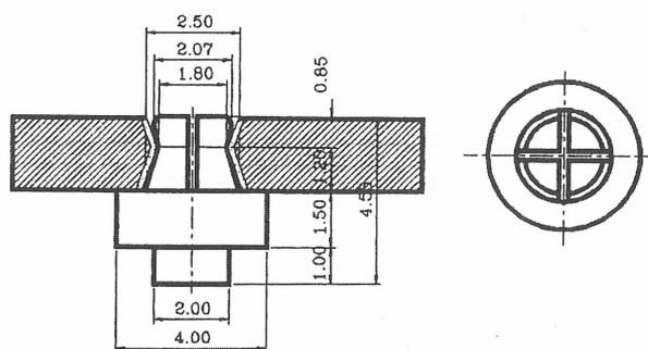
Figure 1 Basic dimensions of the Ceka attachments, measured by a projection profile comparator
