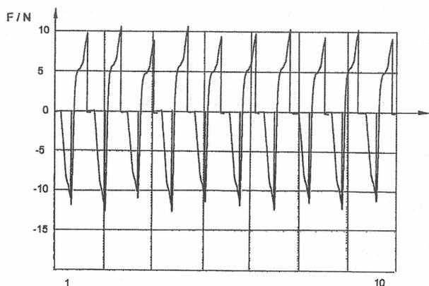
Figure 6 Retention force with added saliva - loading cycles from 1 to 10.
